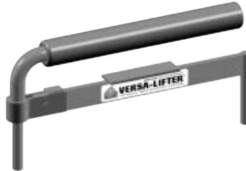
The VERSA-Lifter helps installers construct VERSA-LOK® Standard retaining walls by making it easier to lift and place units — especially on the base course. Two prongs on the Lifter are inserted into pin holes in each VERSA-LOK Standard unit. Lifting the handle secures the Lifter to the unit and makes for easy, balanced lifting and placement.
